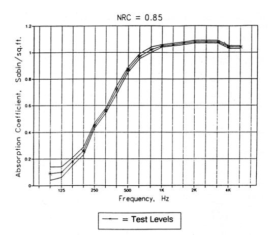
Sound Absorption Coefficient (Sab/ft') vs. Frequency (Hz) on Novawall<sup>TH</sup> 1 Inch Eased Acoustical Panel Assembly
